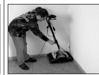
Pull the catch upwards and hold Tip the pushing handle backwards
